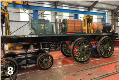
8 & 9: The frames in the process of being lowered onto the wheelsets and bogie...
