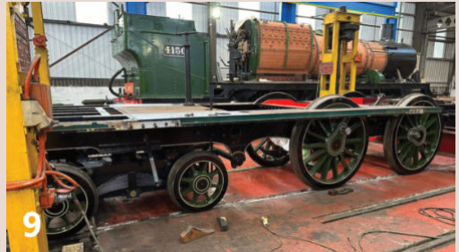
8 & 9: The frames in the process of being lowered onto the wheelsets and bogie...
