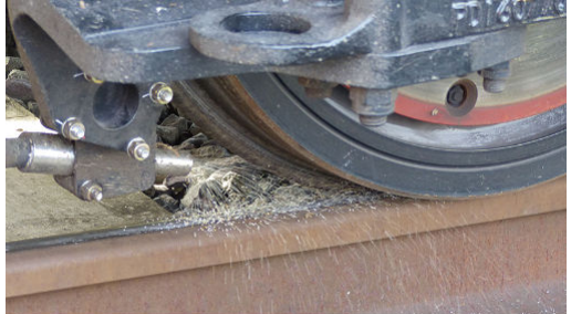
A sander on a class 387 train applying sand to the rail in a static demonstration
