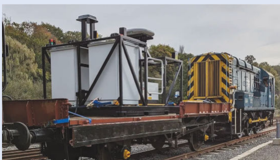
Satellite broadband test rig on North Yorkshire Moors Railway
